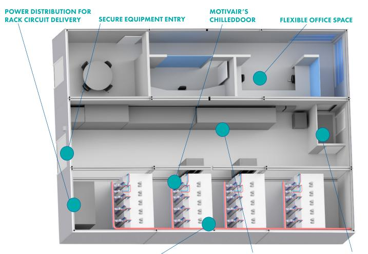
20 EACH 48" DEEP, 50RU IT RACKS WITH REAR DOOR HEAT EXCHANGERS WITH REQUIRED MANIFOLD & CHILLER SYSTEM
